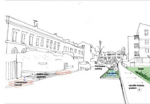
A Create raised entry treatment and geocell storage B Reprofile footway to divert runoff C Make impermeable surfaces permeable
